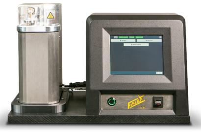
**The instrument is designed for ease of use with automatic operation.** A wide range of retraction speeds, temperatures and probe materials allow for flexibility and customization in identifying adhesion and tackiness properties under a wide range of test conditions. While a 3mm ball stylus is used for standardization work, other materials and geometric shapes are possible.
