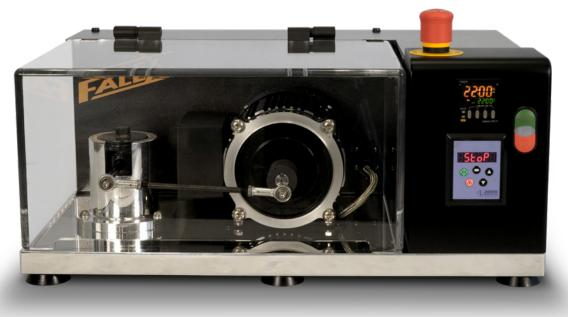
The revamped Fretting Wear Test Machine from Falex meets the requirements of ASTM D4170, "Standard Test Method for Fretting Wear Protection by Lubricating Greases," while offering integrated digital time control, ability to operate at variable speeds, increased user safety and a fresh, modern appearance.
