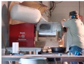
For testing abrasion resistance, Falex Litigation Technical Investigations uses an aggressive test in a dust chamber that was specifically designed to provide repeatable and consistent dust conditions. The dust chamber is configured as a once-through open system. Ambient air is injected via a  $\frac{3}{4}$  hp blower motor and exhausted through a dust capture bag. This permits the air to be circulated around
