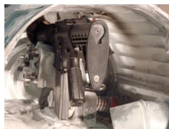
The dust chamber is capable of handling a wide variety of sand/dust types. We have utilized Silica Flour #140 and Silica Sand #35-50, which are materials that meet the specifications of MIL-STD-810F for sand, and rounded quartz grain sand, as typified by AFS 50/70 Test Sand that meets ASTM 65-04 Standard Test Method for Measuring Abrasion Using the Dry Sand/Rubber Wheel Apparatus.
