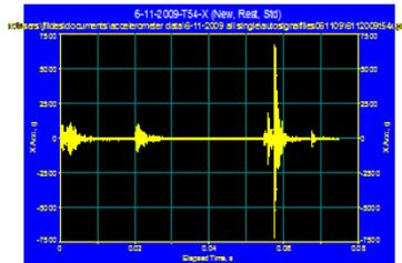
During full-scale testing, the weapon is monitored with a sensor suite that includes a PCB 3 axis accelerometer (model 350B50) that provides a range of +/- 10,000 g's with a frequency response of 10,000 Hz for +/- 1 db and 20,000 Hz for -3 db and a micro-electromechanical (MEMs) acoustic sensor. Data collection is via a National Instruments USB
