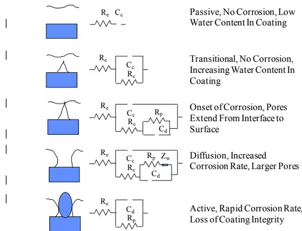
The fourth method we use is also an alternating current (ac) method that is relatively recent. It provides an uncontaminated value of the corrosion current, as well as of the Tafel coefficients, without requiring use of large dc potentials that can alter the surface of the electrode, and it does not require extensive modeling, but also does not provide mechanistic insight.
