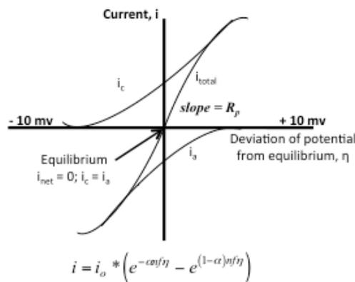
Measuring the slope,  $R_p$ , of line obtained in the “Linear Polarization” plot provides the corrosion current, but quantities called the Tafel coefficients,  $B_a$  and  $B_c$ , are required for this computation. The Tafel coefficients are often assumed to have certain values, but this causes an error whose extent is unknown and that can be large.
