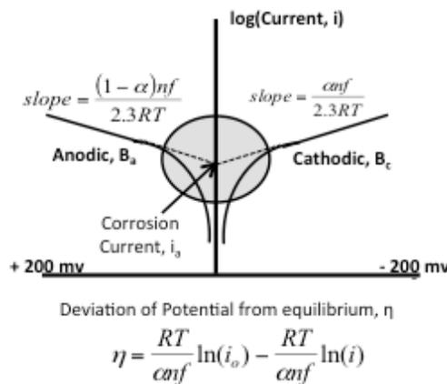
Each branch shows a linear portion and extrapolation to the free corrosion potential provides the corrosion current at the free corrosion potential. The slopes of the anodic and cathodic lines are the Tafel coefficients. The problems with this approach are that large potentials can sometimes drive unwanted reactions that obscure the linear portion of the anodic or cathodic branch, making extrapolation inaccurate, and irreversibly altering the electrode surface.
